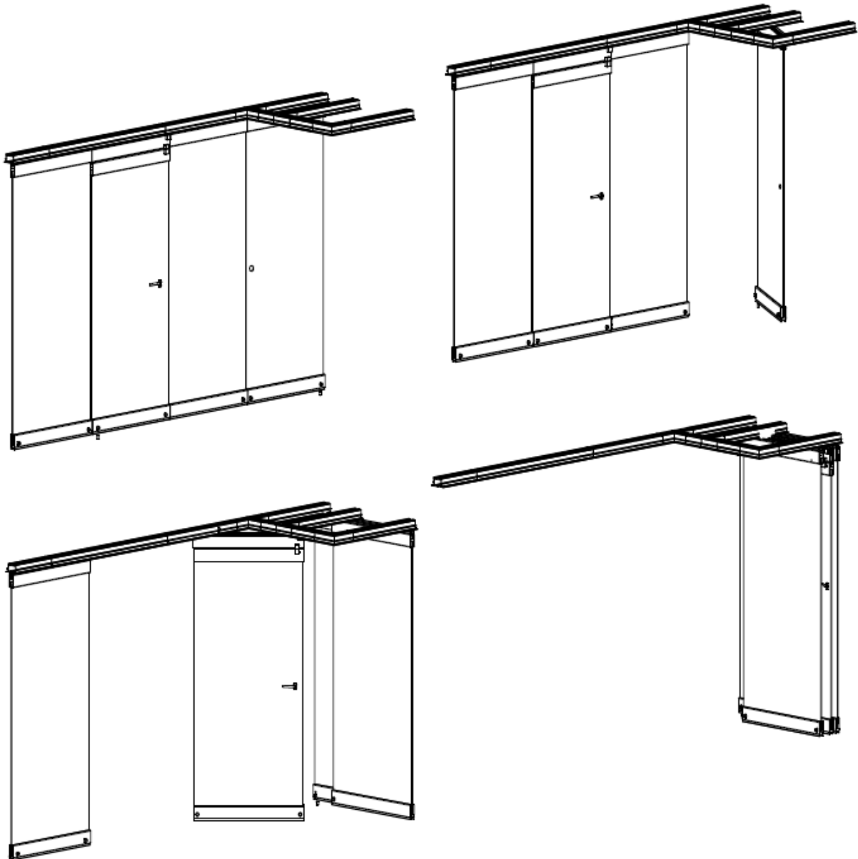
Fig.7 The idea of handling an all-glass wall in a 2-point panel suspension system (panels are parked in parking racks)
